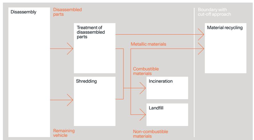
In the disassembly stage, hazardous and/or valuable components are removed from the vehicle including:
